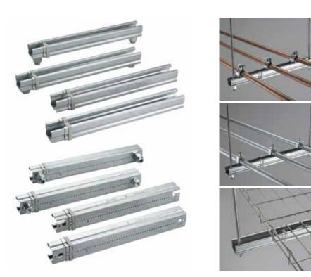
The Telescoping Strut Replacement is an innovative alternative to using traditional strut channels for trapeze or other support structures that accommodates standard strut fittings. This telescoping solution eliminates the need to handle and cut long lengths of strut to size. The bracket telescopes to the desired length and is locked in place by snapping closed a spring retainer clip.
